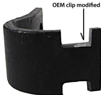
**1/8" of clip slot removed for thicker SuperCoil installation**
