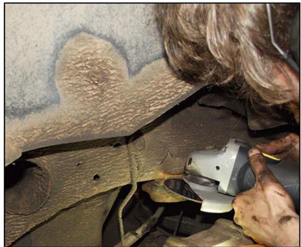
Remove factory bumpstop bracket by grinding the weld off or by using a heavy hammer and chisel to remove the tack weld.
