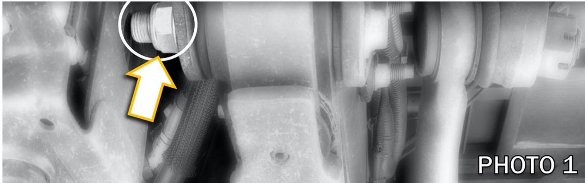
Remove the nut (**PHOTO 1**) from the forward spring eye bolt (15/16 wrench for nut)(13/16 or 21mm for bolt head)
