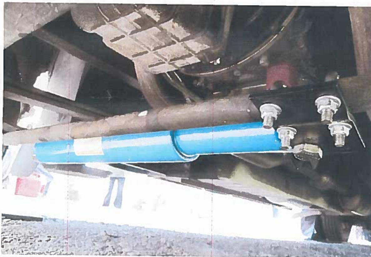
Completed installation of Safe-T-Plus Steering Control on Straight Axle.
