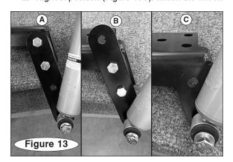
absorber to whichever mounting hole on the tie plate is more appropriate as described below.
