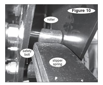
Finish with a 7/16" nylock nut and torque to 40 lb-ft.
