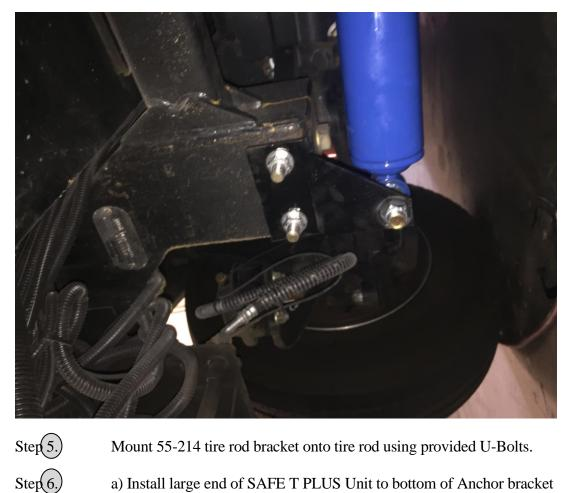
b) Install small end of SAFE T PLUS unit to bottom of Tie Rod Bracket with bolt, nut, & washer provided.
