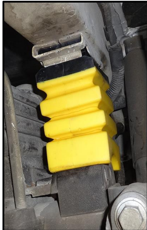
Equipped with 2" axle spacer
